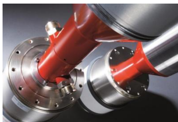
Fig. 1. High-power motorized vacuum capacitors (100-1600 pF, 3-30MHz, 30 kV peak,working , 800 Arms)
