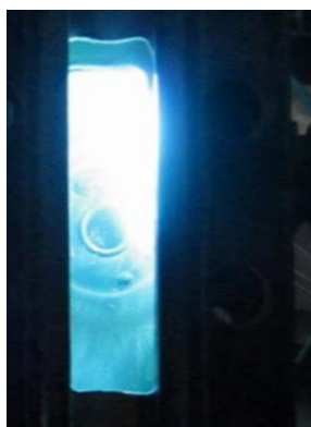
Fig. 1. The transonic flow (directed upwards, particle velocity u=350 m/sec before start of combustion)
