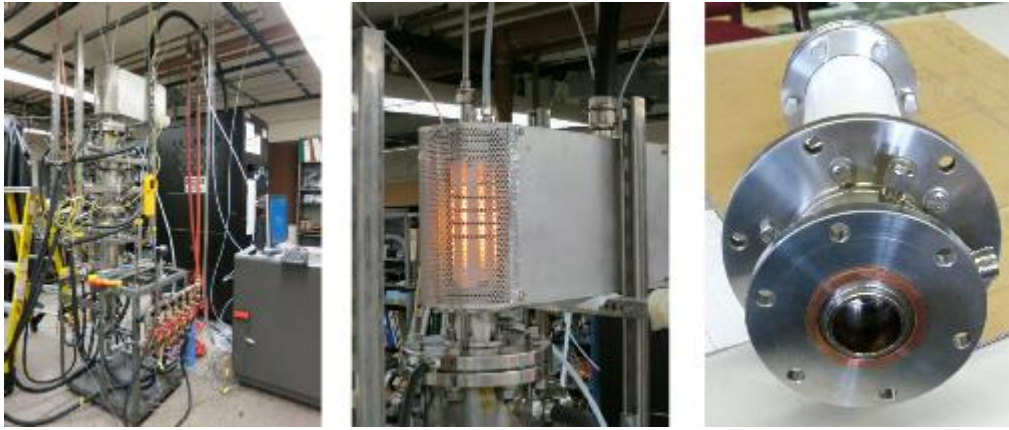
Fig. 2. From left to right: general view of experimental setup, vertically positioned torch in operation, plasma torch integrated with a powder feeding nozzle
