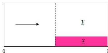
Fig. 1 Scheme of local air heating in the scramjet channel. The arrow shows flow direction.
