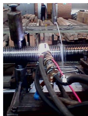
Fig. 4. Hardening of a bifilar trapezoidal lead screw thread for turning lathe \varnothing 120 mm, 5,500 mm long, made of 45 steel
