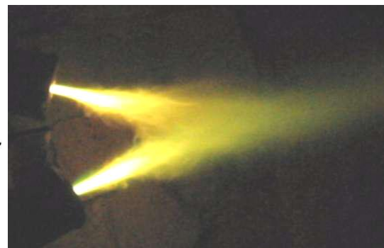
Fig. 1. Schematic and operating view for the investigated twin plasma torch.
