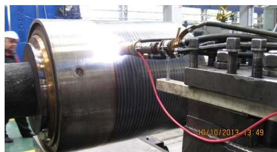
Fig. 2. Hardening of a batch of rolling mill bearing shells made of 45 steel, with pressed bronze sleeves
