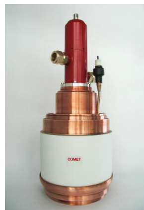
Fig. 2: Example of a customized variable vacuum capacitor for RF heating (15-150 pF, 40-55 MHz)
