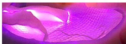
Fig. 4. Porous surface in RF capacitive discharge at reduced pressure
