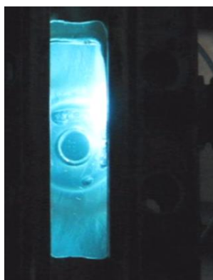
Fig. 2. The supersonic flow (directed upwards, particle velocity u=540 m/sec before start of combustion)
