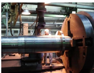
Fig. 1. Hardening of spindle collars for heavy turning lathe made of 35HN3MFA steel, 6,500 mm long, with the weight of 10,850 kg
