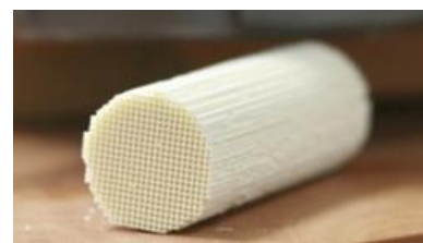
Fig. 1. A cylindrical cut from cordierite catalytic block
