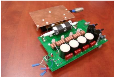
Fig. 1. Nanosecond pulsed discharge unit for internal combustion engines
