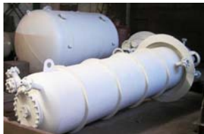
Fig. 5. Melting and halogen removal devices
