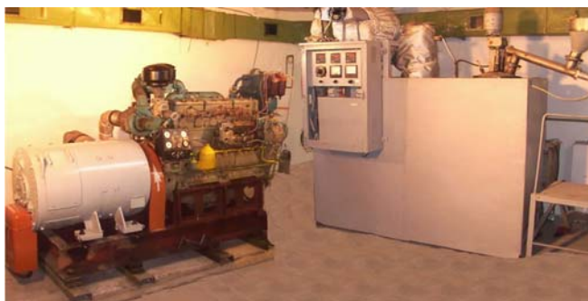
Fig. 3. Experimental facility for thermoplastic waste processing into fuel
