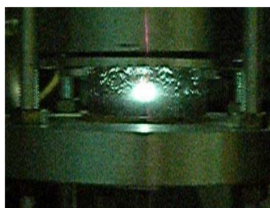
Fig. 4. Discharge pictures at constant flow of air in ethanol
