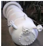
Fig. 5. Melting and halogen removal devices
