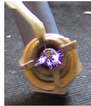
Fig. 2. Multiple streamers produced by the PDI.
