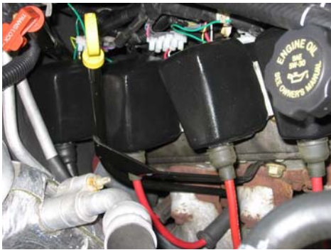
Fig. 1. PDI units with misfire detection feedback mounted on a late model GM vehicle.
