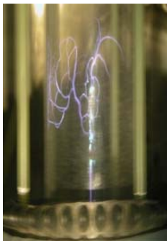
Fig. 3. Subcritical streamer MW discharge in a reverse vortex combustor
