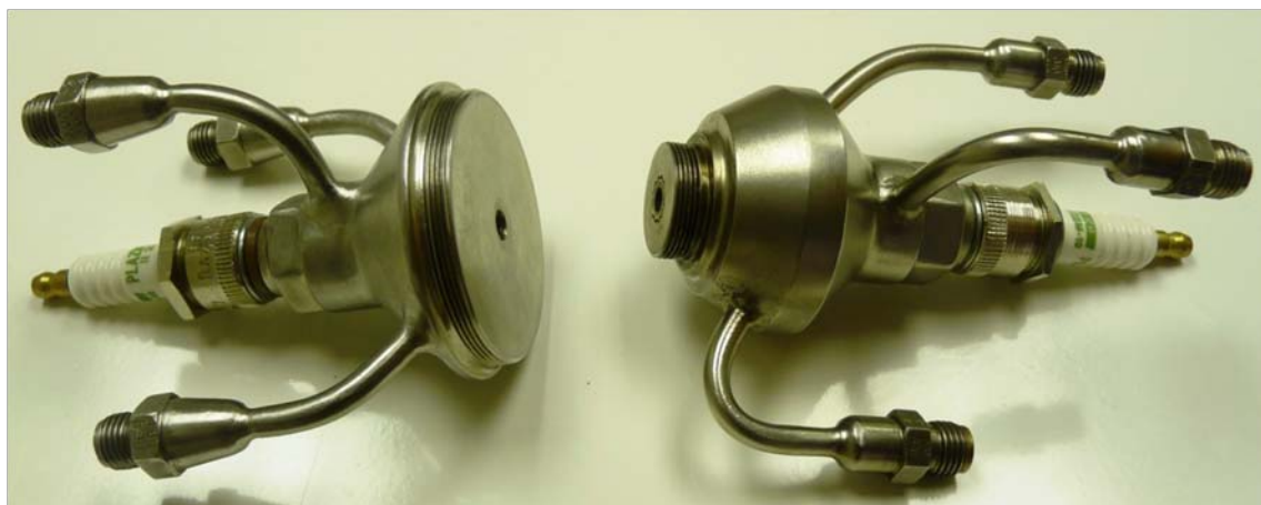
Fig. 1. PFN modifications with the cross flow channels
